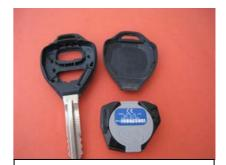
Separate back part of the cover from the key and remove electronic board.
