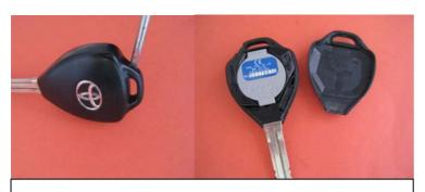
Position flat screwdriver in a small slot at the top of your remote and twist it, so detachable part moves away from key part.
