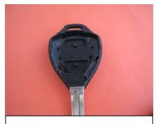
Place electronic board back in remote, cover it with bottom part of the shell and close it.
