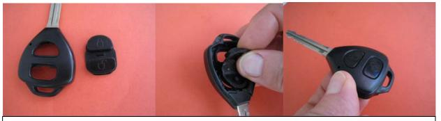
Silicone buttons will be fitted from inside of the remote. Simply press fit silicone buttons in. Make sure that buttons are fitted flat with the surface of the plastic shell.
